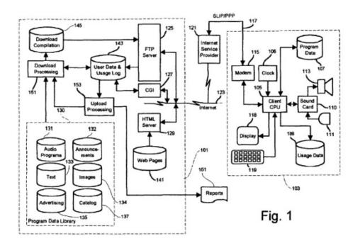
Although described as a "Host Computer" in the dashed line, this term is used loosely, as each of the claimed components is shown individually attached to the Internet.
