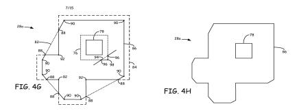
Fig. 4G and Fig. 4H show how the inwardly offset convex hull and the boundary polygon are merged to created the "intersection boundary polygon" in Fig. 4H, which is essentially a smoothed, inwardly offset shell that fits inside the original boundary polygon.
