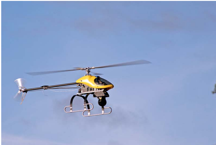
Photo1: Electric rotary wing Maxi Joker 2 with autopilot and gimbaled camera system.
