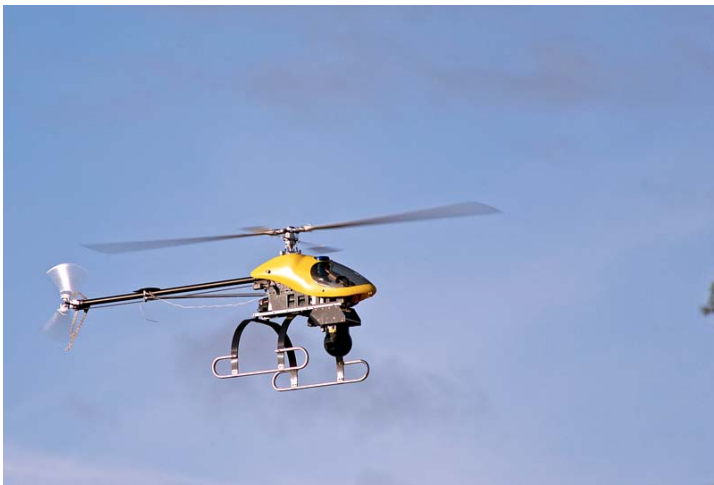
Figure 3: Electric rotary wing Maxi Joker 2 with autopilot and gimbaled camera system.
