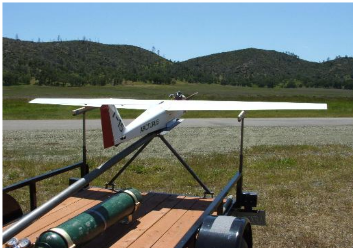
Photo 1: Pneumatic Launcher for T15/T16
