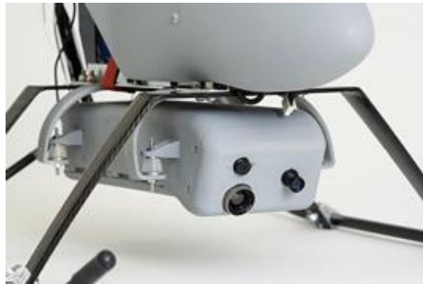
Fig 2. The avionics box housing the FCS20 and camera system
