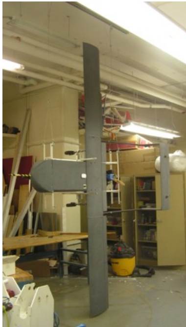
Figure 12: Measuring inertia: SPAARO suspended from two filaments.
