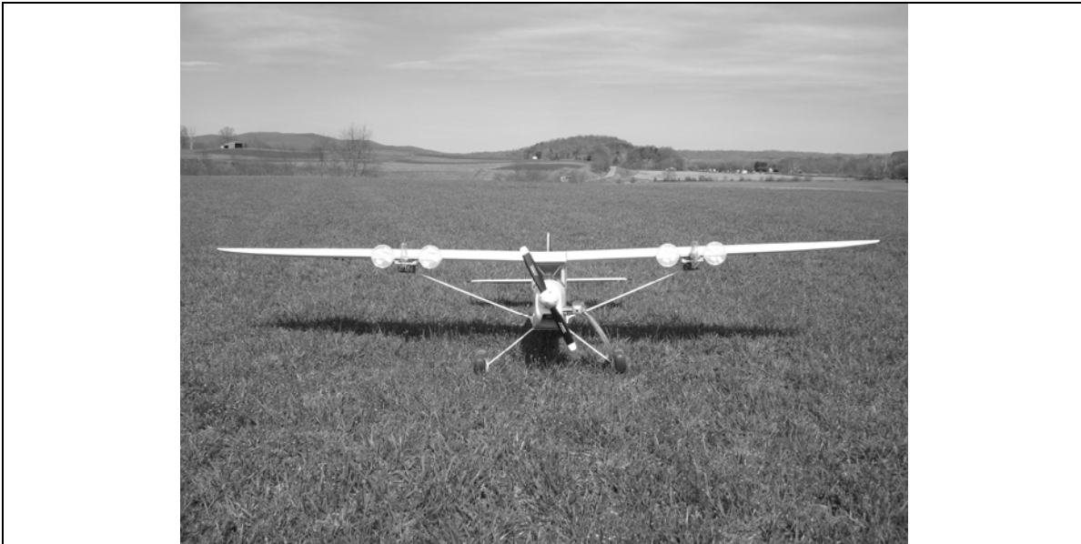
FIGURE 2. Aerobiological sampling devices mounted underneath the wings of the Rascal 110 UAV. The sampling devices are closed during takeoff and landing, and opened when the UAV reaches its target sampling altitude.
