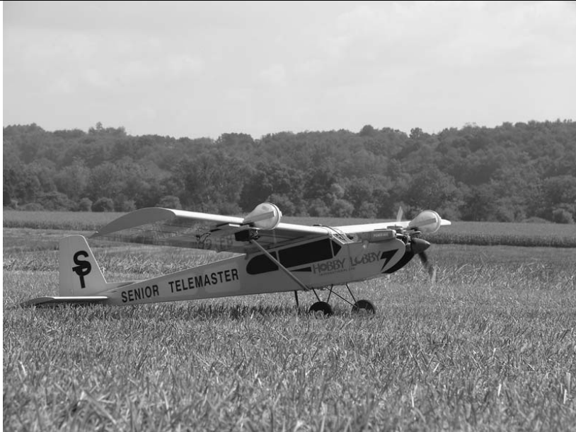
FIGURE 1. ST UAV with aerobiological sampling devices mounted in front of the leading edge of the wings.
