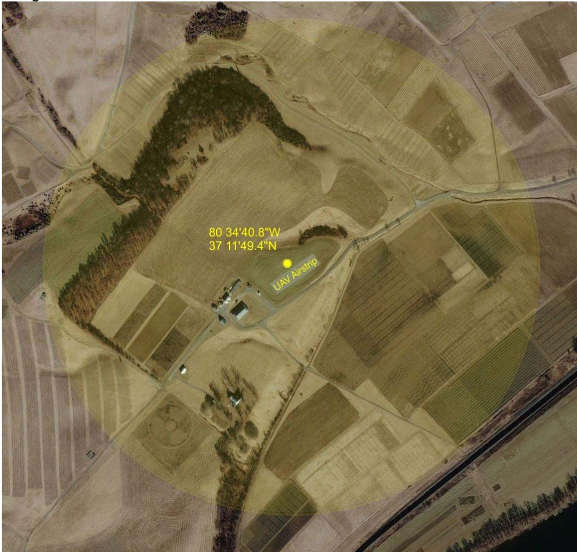
**Specified flying area at the Kentland Farm:** A circle (shaded yellow) of one-quarter mile radius, centered at 80:34'40.80\"W and 37:11'49.40\"N. The UAV will never be more than 1500 feet from the UAV airstrip, which is located on a hilltop, offering unobstructed views of the operating area. There are no public roads through or near the Kentland Farm.
