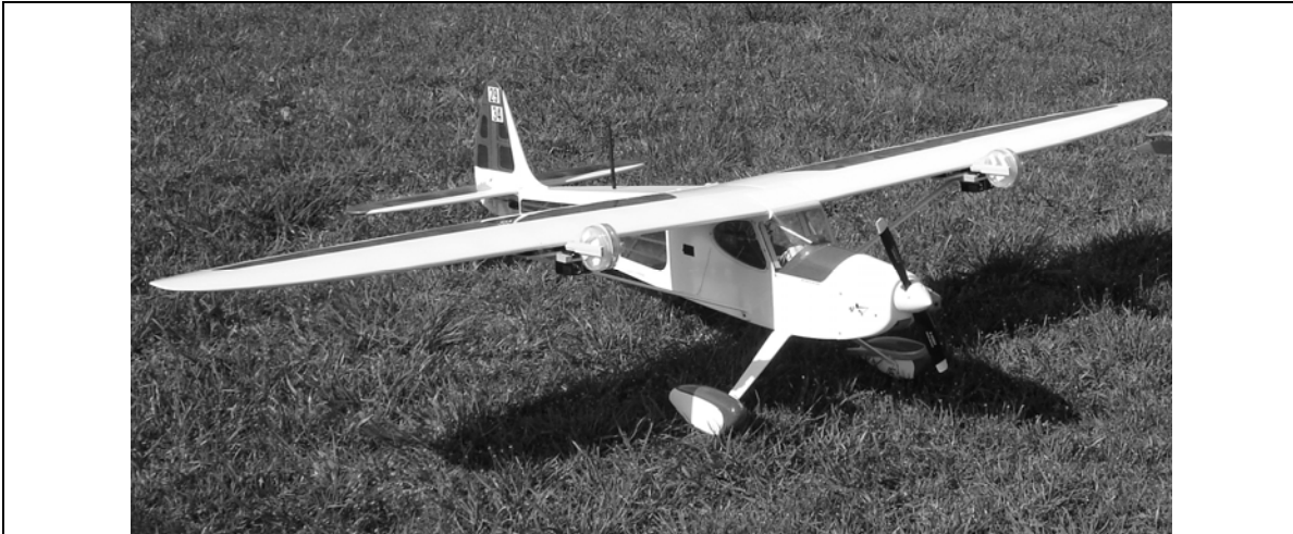
FIGURE 1. Rascal 110 UAV with aerobiological sampling devices mounted in front of the leading edge of the wings.
