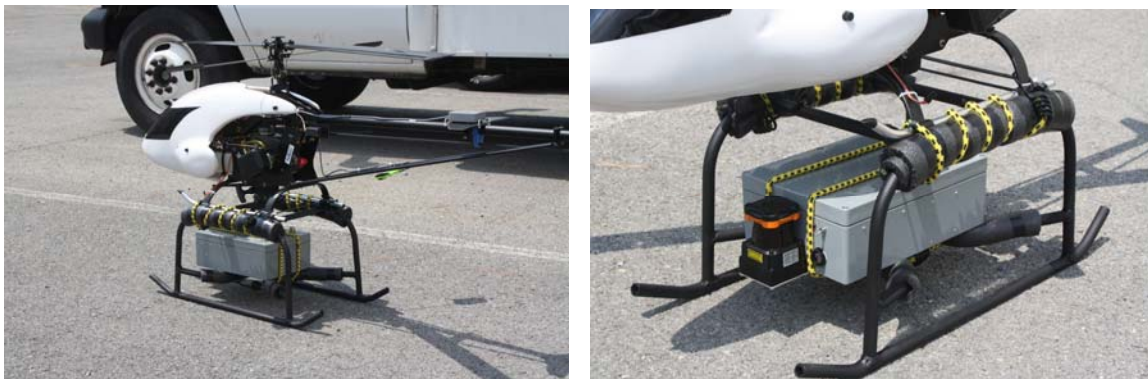
Figure 4: Payload Carrier and Sensor Payload Mounted to the Bergen Helicopter.
