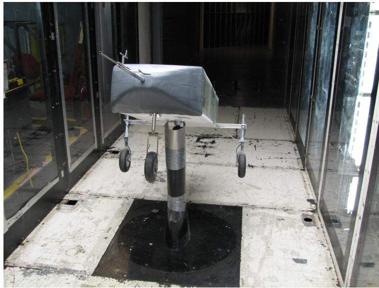
Figure 9: SPAARO Air Data Boom Calibration in VT's Stability Wind Tunnel
