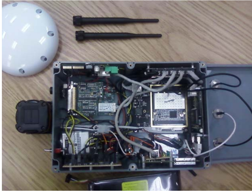
Figure 3: Antennas and Internal View of Sensor Package. Battery has been Removed to Facilitate Viewing Internal Components.
